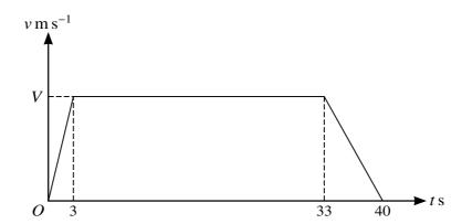
The diagram shows the velocity-time graph of the journey of a bus between two bus stops P and Q. The bus starts from rest at P and accelerates at  $4 \,\mathrm{m \, s^{-2}}$  for  $3 \,\mathrm{s}$ . The bus continues at constant speed,  $V \,\mathrm{m \, s^{-1}}$ , for a further  $30 \,\mathrm{s}$ . Then the bus decelerates uniformly for  $7 \,\mathrm{s}$  until it reaches Q. Find
